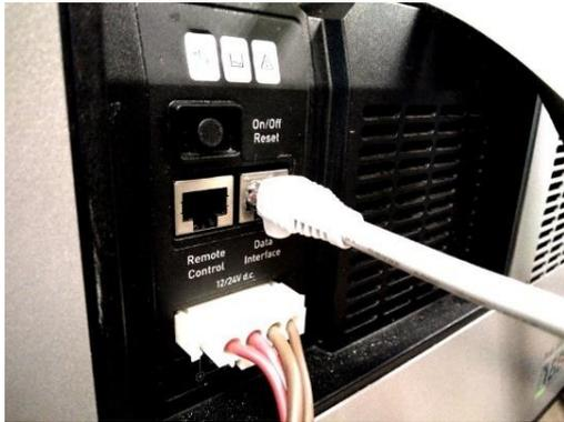
Connect the Data Cable to the Fuel Cell using the Data Interface Port on the unit.
