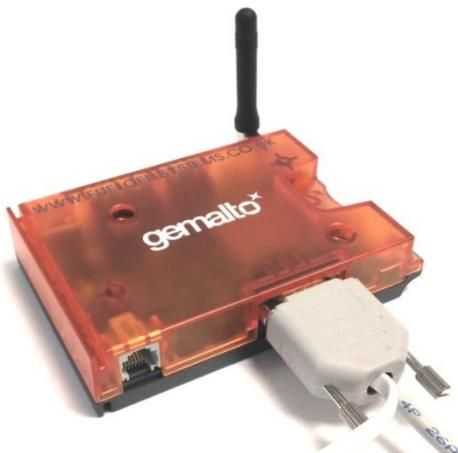
Connect the Data Cable to the 3G Modem
