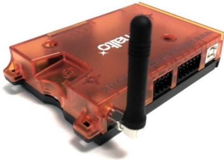
Connect the Antenna to the 3G Modem
