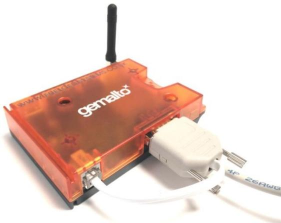
Connect the Power Cable to the 3G Modem
